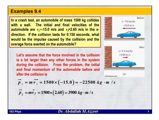
Therefore the impulse on the automobile due to the collision is  $\vec{I} = \Delta \vec{p} = \vec{p}_{,-} - \vec{p}_{,i} = (3900 + 22500) \ kg \cdot m / s \\ = 26400 \ kg \cdot m / s = 2.64 \times 10^4 kg \cdot m / s$  The average force exerted on the automobile during the collision is  $\vec{F} = \frac{\Delta \vec{p}}{\Delta t} = \frac{2.64 \times 10^4}{0.150} = 1.76 \times 10^5 \ N$  Read the rest of the example
