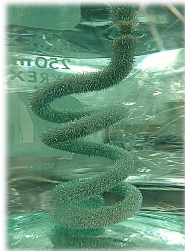
Photograph of a “silver tree” created by immersing a coil of copper wire in a solution of silver nitrate.
