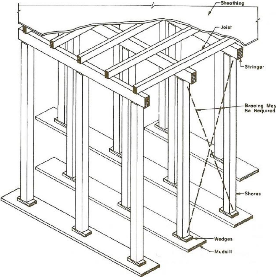
**FIGURE 12-22: Beam and slab form.**
