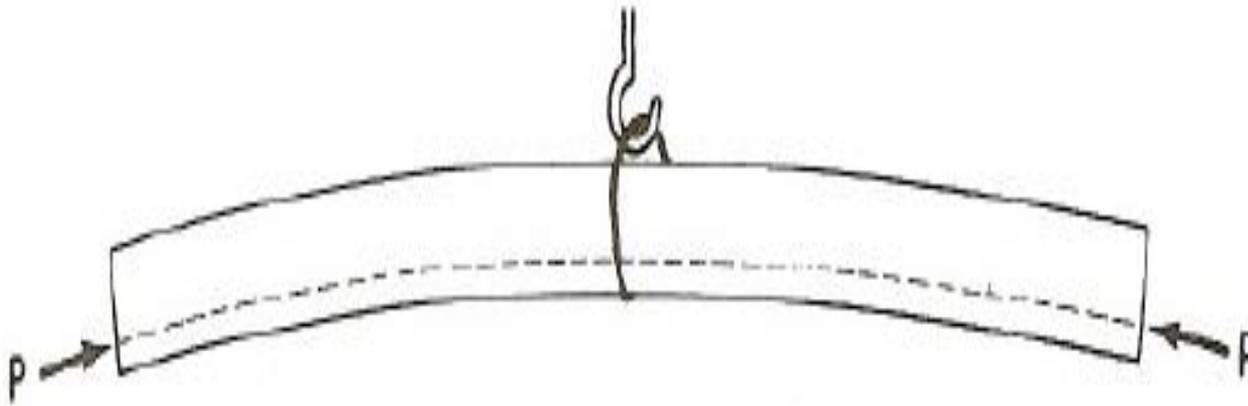
FIGURE 12-11: Lifting prestressed beam at the center.
