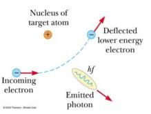
The maximum x-ray energy, and minimum wavelength results when the electron loses all its energy in a single collision, such that
