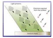
Increasing the brightness of the light did not eject faster electrons - think of light as a wave - brighter light (bigger amplitude wave) should eject more energetic (faster) electrons.
