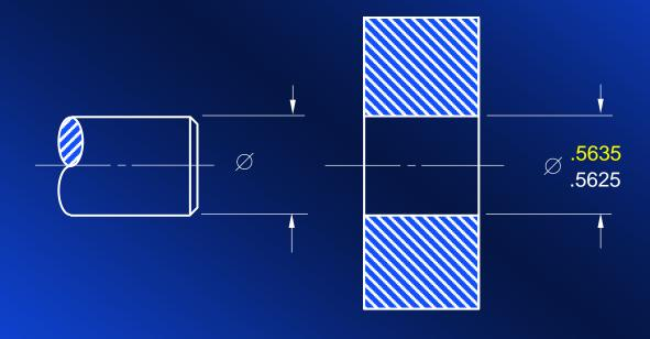
To determine the upper size limit of the shaft, we must subtract (note the sign in the table for the upper size limit of the shaft) 0.6 thousandths (or six tenthousandths) from the basic size. The result will be .5619 (.5625 - .0006 = .5619). Add this value to the drawing as the upper size limit on the shaft.
