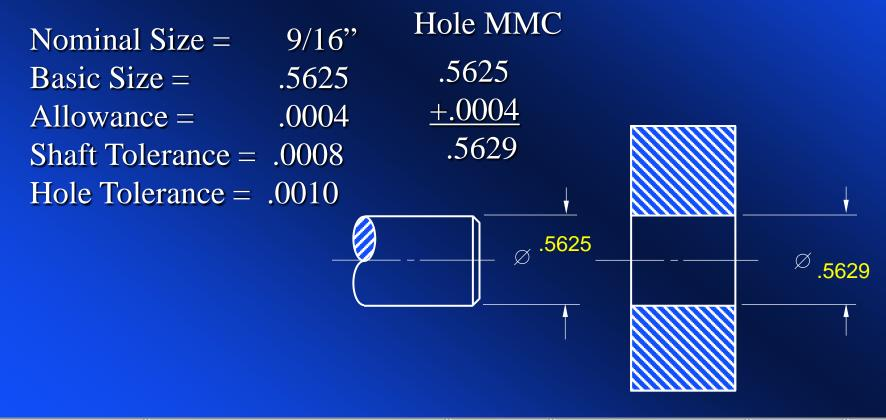
The process is completed by applying the tolerances to the respective components by subtracting the shaft tolerance from the shaft upper limit, and adding the hole tolerance to the hole dimension lower limit. Apply your results to the drawing.
