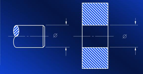
The first column for a class RC 4 fit establishes the *limits of clearance*. The number on top is the *allowance* at MMC. Converted to inches (by moving the decimal 3 places to the left), this number would be .0006, six tenths of one-thousandth, or six ten-thousandths. The number below (2.3) is the maximum clearance at LMC, or twenty-three ten-thousandths (.0023).
