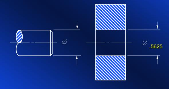
For the upper size limit for the hole you will notice that the value on the chart is +1.0. This value when converted into inches equals one thousandth of an inch — or ten ten-thousandths. Add the required .0010 to the basic size for the upper limit of the hole (.5625 + .0010 = .5635). This is the upper size limit of the hole, which can now be added to the drawing. *It is added to the basic size value.*
