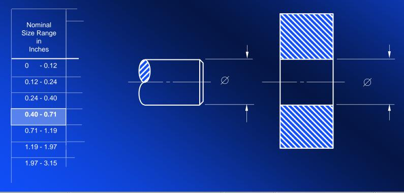
Next, read across the table on the row that is highlighted to identify the parameters for an RC 4 fit. Because of the lack of space, the columns for fits other than the RC 4 are excluded.
