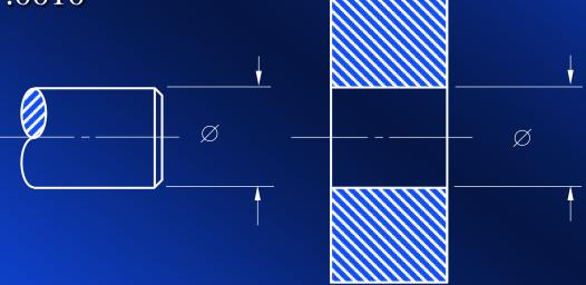
The basic shaft system establishes the basic size as the maximum shaft size. Remember, the upper size limit *always* goes on top in a stacked tolerance expression.
