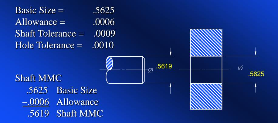
Apply the *tolerances* to both the hole and the shaft to complete the dimensions; *add* the hole tolerance to the hole lower limit, and *subtract* the shaft tolerance from the shaft upper limit. Do the arithmetic and apply the values.
