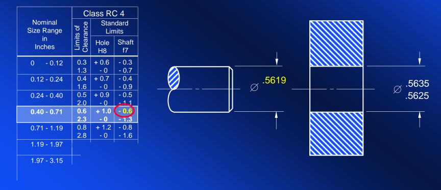
Finally, determine the lower limit of the shaft diameter by subtracting 1.3 thousandths (or thirteen ten-thousandths) from the *basic size*, and include the value in the drawing.
