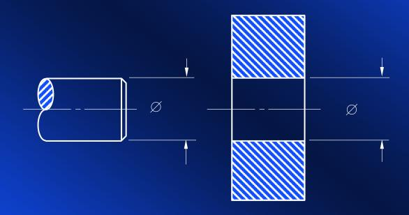
First, identify the size range in the left-most column in the fit table for RC fits. The row that identifies the size range that will include the designated diameter in the problem have been highlighted. Note that this column is specified in inches. All other columns in the table are specified in *thousandths* of an inch.
