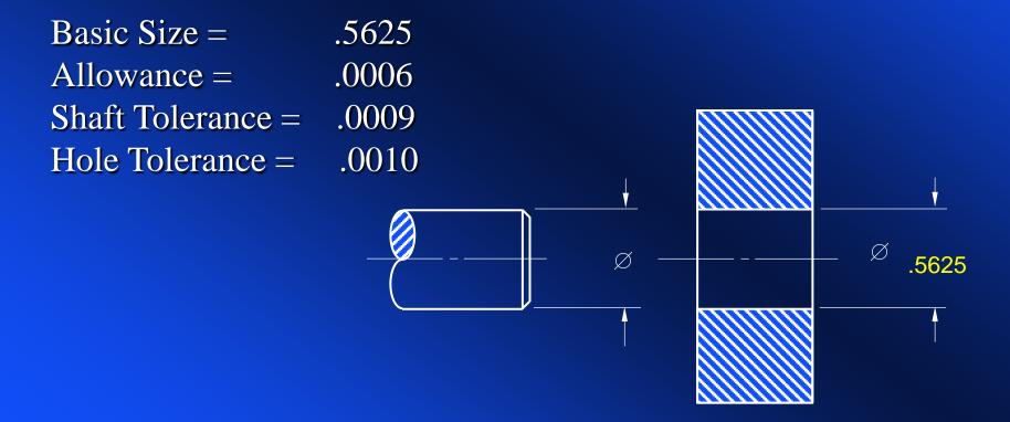
Subtract the *allowance* from the basic size to obtain the maximum shaft size (Shaft MMC). Place the value as the upper limit of the shaft dimension.
