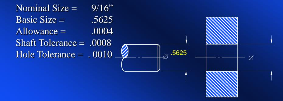
The minimum hole size (Hole MMC) is obtained by *adding* the allowance to the basic shaft size. Do the addition and place the dimension as the lower limit of the hole size.
