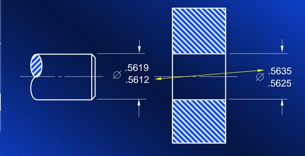
Values Referenced to Basic Size:  $\varnothing$  .5625  $\stackrel{\text{-.0006}}{\text{-.0013}}$
