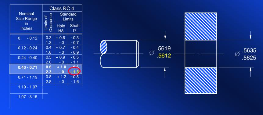
Now, look back to the column labeled "Limits of Clearance". These values reveal the total amount of variation that can be allowed on a 9/16" RC 4 fit—when the parts are at maximum material condition and at least material condition.
