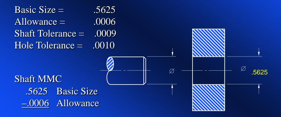
Subtract the *allowance* from the basic size to obtain the maximum shaft size (Shaft MMC). Place the value as the upper limit of the shaft dimension.
