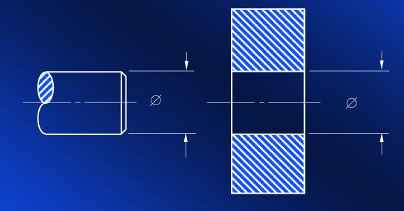
Notice that the *Hole* size, at its *lower* limit, reads "- 0". Therefore, use the basic size (nominal 9/16 inch, converted to its decimal equivalent, .5625) as the lower limit for the dimension of the hole.
