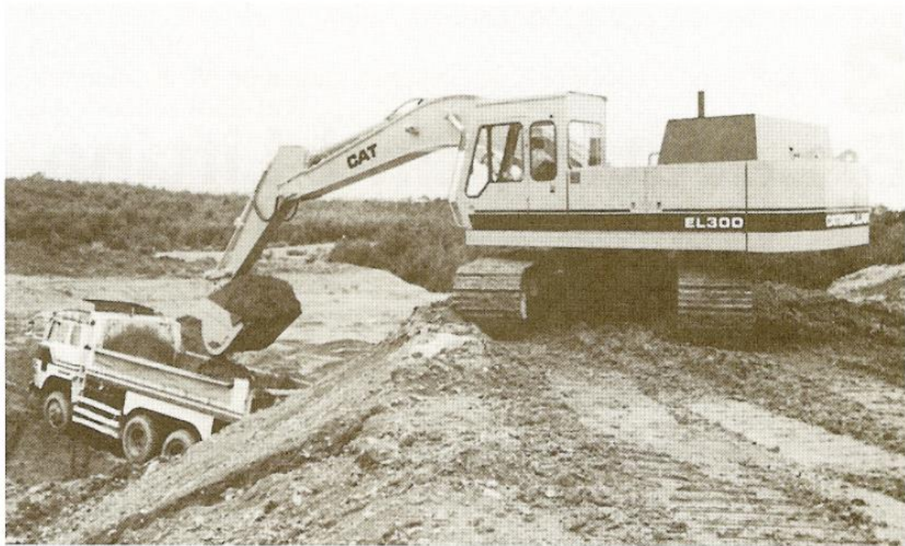
FIGURE 3-1 Hydraulic excavator-backhoe. (Courtesy of Caterpillar Inc.)
