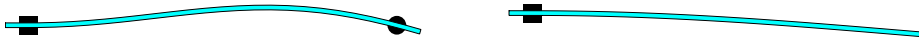
Fig. 1. The depicted boundary condition for the left endpoints of these two cross sections is clamped , while the boundary conditions for the right endpoints are respectively hinged and free .
