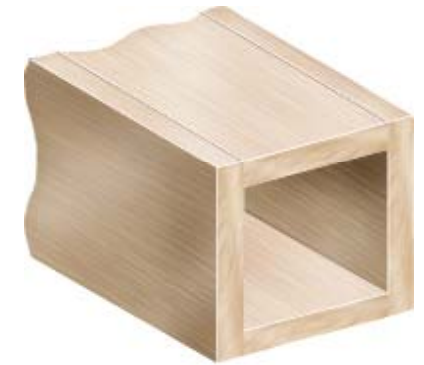
Wooden box beam
