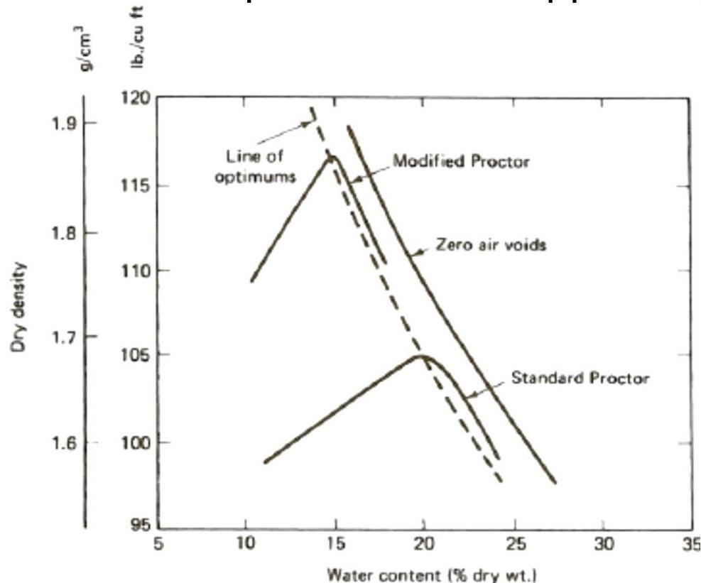
FIGURE 5-1: Typical compaction test results.
