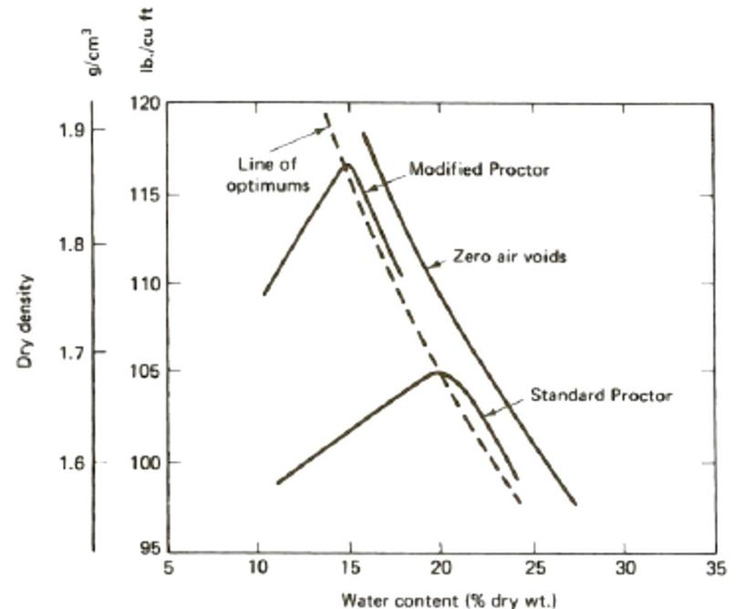
**FIGURE 5-2: Modified Proctor Test results for various soils. (Courtesy of Dr. Harvey E. Wahls)**
