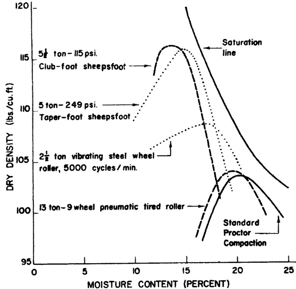
THE EFFECT OF MOISTURE CONTENT ON THE DRY DENSITY OF A SILTY CLAY (CL) SOIL IN 9 in. LOOSE LAYERS WHEN FULLY COMPACTED BY UP TO 64 PASSES BY DIFFERENT TYPES OF COMPACTING EQUIPMENT.
