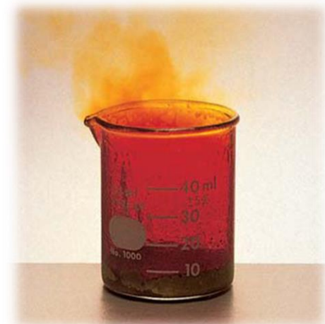
Aluminum reacting with bromine to form aluminum bromide
