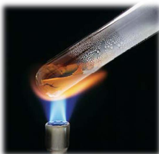
On heating, mercury(II) oxide (HgO) decomposes to form mercury and oxygen
