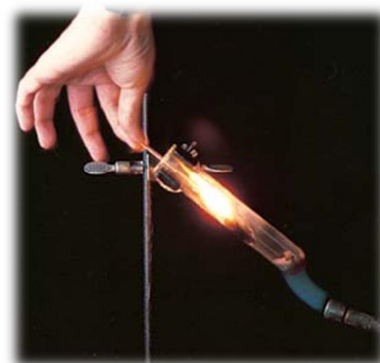
Heating potassium chlorate (KClO 3 ) produces oxygen, which supports the combustion of the wood splint
