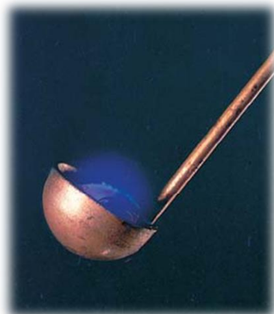
Sulfur burning in air to form sulfur dioxide
