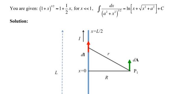
We consider the elementary part  $d\mathbf{l}$  of the wire at a position x having length dx. Thus  $d\mathbf{l} = dx\hat{\mathbf{x}}$ . This part is flown by a current I so at the point  $P_1$  it creates a vector potential  $d\mathbf{A}$  given by:
