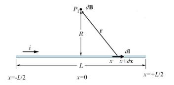
To solve this problem we need to apply Biot-Savart Law. We consider the elementary part  $d\mathbf{l}$  of the wire at a position x having length dx. Thus  $d\mathbf{l} = dx\hat{\mathbf{x}}$ . This part is flown by a current I so at the point  $P_1$  it creates a magnetic field  $d\mathbf{B}$  given by:
