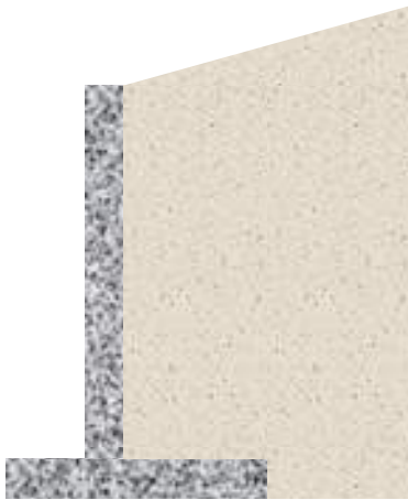
Cantilever retaining wall
