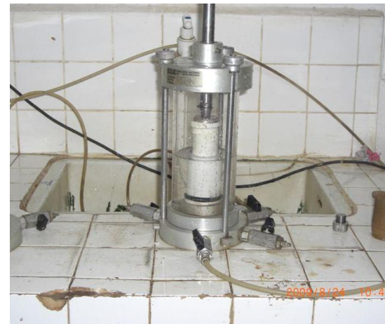
Cell is completely filled with water
