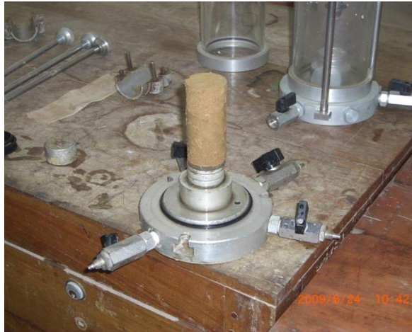
Setting up the sample in the triaxial cell
