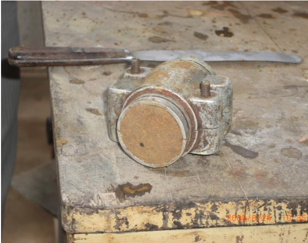
Edges of the sample are carefully trimmed
