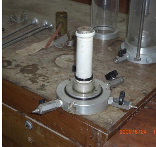
Sample is covered with a rubber membrane and sealed
