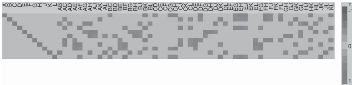
■ FIGURE 9.17 Correlations of main effects and two-factor interactions, no-confounding design for 11 factors in 16 runs
