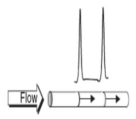
Open tube, inner diameter: 50-150 µm
