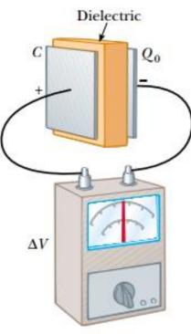
Capacitance of a capacitor filled with a material of dielectric
