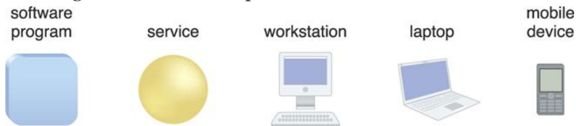
Figure 3.7. Examples of cloud service consumers. Depending on the nature of a given diagram, an artifact labeled as a cloud service consumer may be a software program or a hardware device (in which case it is implied that it is running a software program capable of acting as a cloud service consumer).
