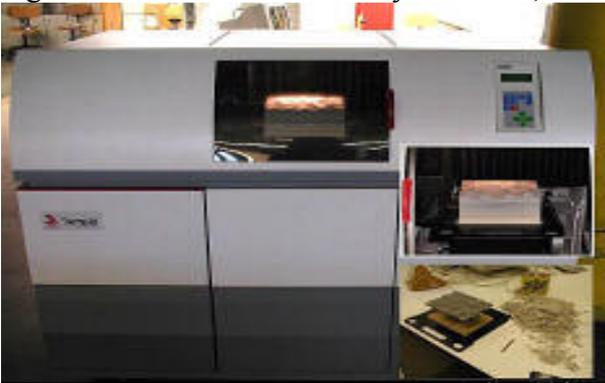
Figure 13. Taking Sketching and Concept-Development One Step Further By Transforming Concepts Into Tangible Prototypes. Rapid Prototyping And Stereolithography<sup>28</sup> Using A Thermojet Printer. Students build physical models directly from their Rhino files. (The top insert shows the build chamber while the bottom shows a model during the cleaning process to remove supports.)
