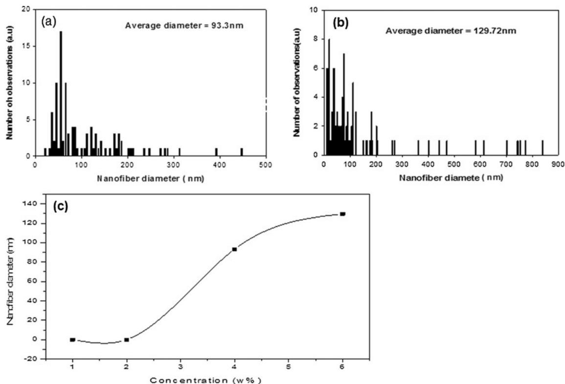
**Fig. 1** Effect of chitosan solution concentration on the diameter distribution of NFs at constant applied voltage, flow rate, tip to collector distance, and needle diameter: **a** 4 wt% histogram, **b** 6 wt% histogram, **c** sigma plot of the same
