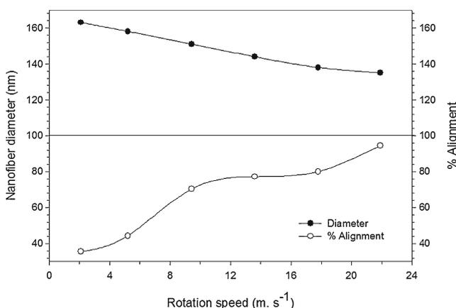
**Fig. 3** Effects of rotation speed on alignment and diameter of the chitosan NFs
