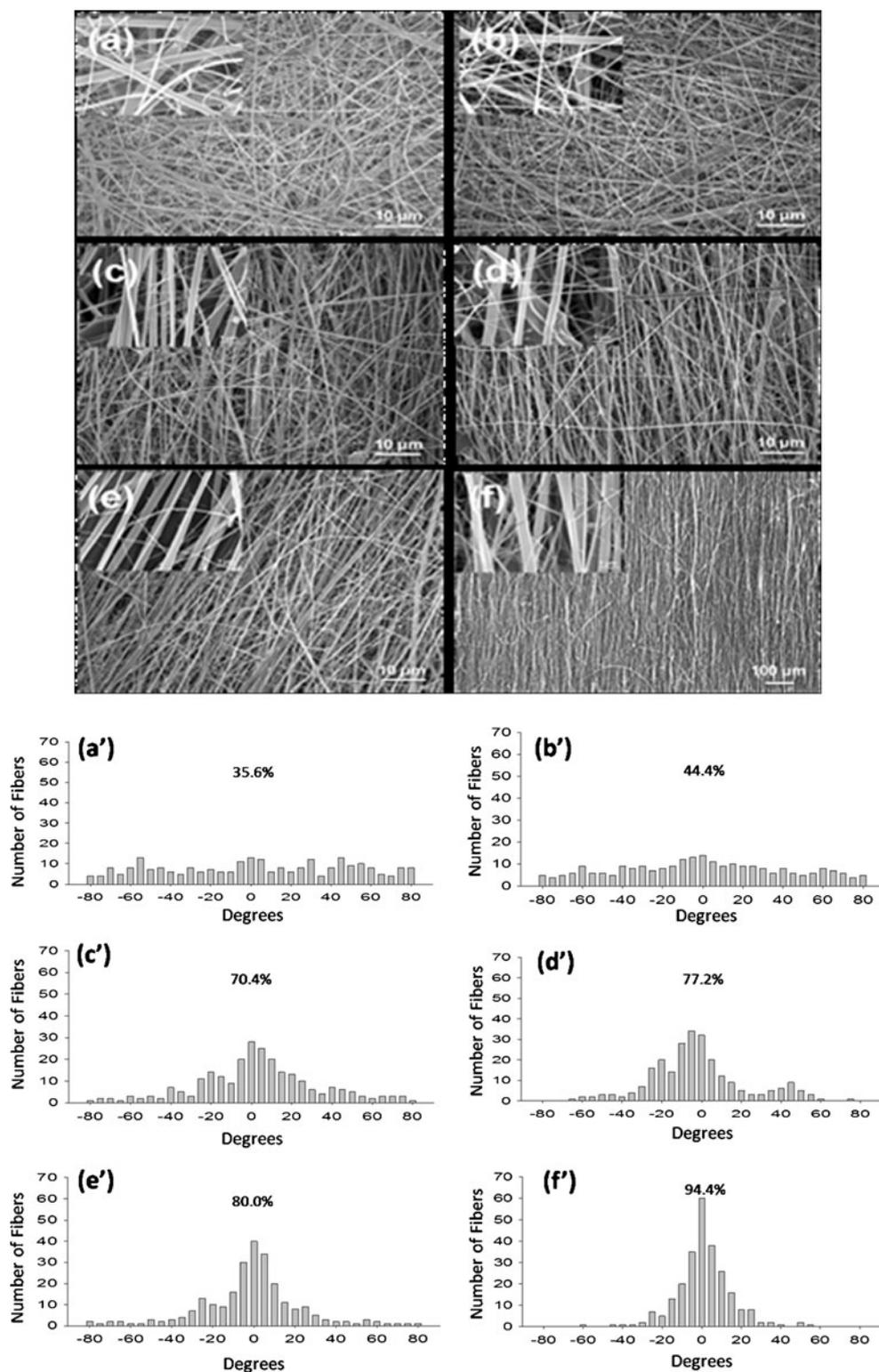
and randomly aligned NFs on the collector plate. The technique was, however, successful in obtaining aligned NFs for a very short time of 30 s [25]. More recently Khamforoush and Mahjob [26] designed a modified rotating jet technique (Table 3, inset e) to increase the amount and degree of alignment of the PAN nanofibers. The cylindrical collector of the
