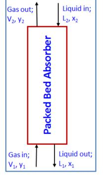
(5) For a given separation in a counter-current packed bed absorber, if  $x_1, y_1$  are in equilibrium, then the absorber
