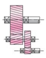
A gearbox is needed to provide an *exact* 30:1 increase in speed, while minimizing the overall gearbox size. Specify appropriate teeth numbers.
