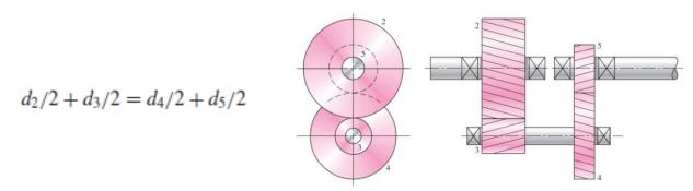
The diametral pitch relates the diameters and the numbers of teeth, P = N/d. Replacing all the diameters gives
