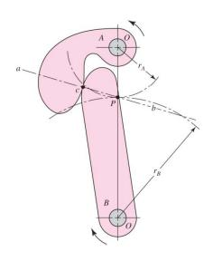
Mating gear teeth produce rotary motion similar to cams
