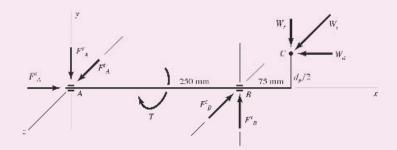
These three forces,  $W_r$  in the -y direction,  $W_a$  in the -x direction, and  $W_t$  in the +z direction, are shown acting at point C in Fig. 13–39. We assume bearing reactions at A and B as shown. Then  $F_A^x = W_a = 74$  N. Taking moments about the z axis,
