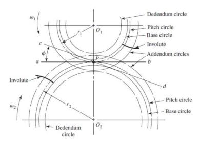
Next, on each gear draw a circle tangent to the pressure line. These circles are the *base circles*. Since they are tangent to the pressure line, the pressure angle determines their size. As shown in Fig. 13–10, the radius of the base circle is
