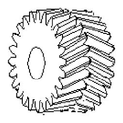
Herringbone gears are mostly used on heavy machinery.
