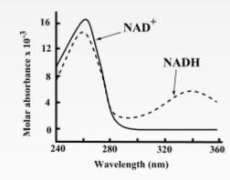
The absorbance at **340nm** is measured each minute without stopping the reaction, resulting in **decreased** readings **due to the oxidation of NADH.**
