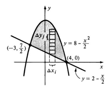
$$A = \int_{-3}^{4} \int_{2-(x/2)}^{8-(x^2/2)} dy \, dx = \int_{-3}^{4} \left[ \left( 8 - \frac{x^2}{2} \right) - \left( 2 - \frac{x}{2} \right) \right] dx$$
