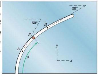
$$2/65 \quad v = \dot{s} = \frac{t}{2} \quad v_{A} = \frac{2}{2} = 1 \, \text{m/s}, v_{B} = \frac{2.2}{2} = 1.1 \, \text{m/s}$$
