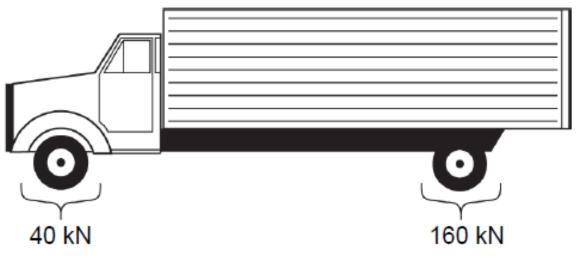
Ex: Contact Force between a wheel and ground.
