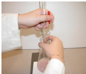
The correct way of handling a burette
