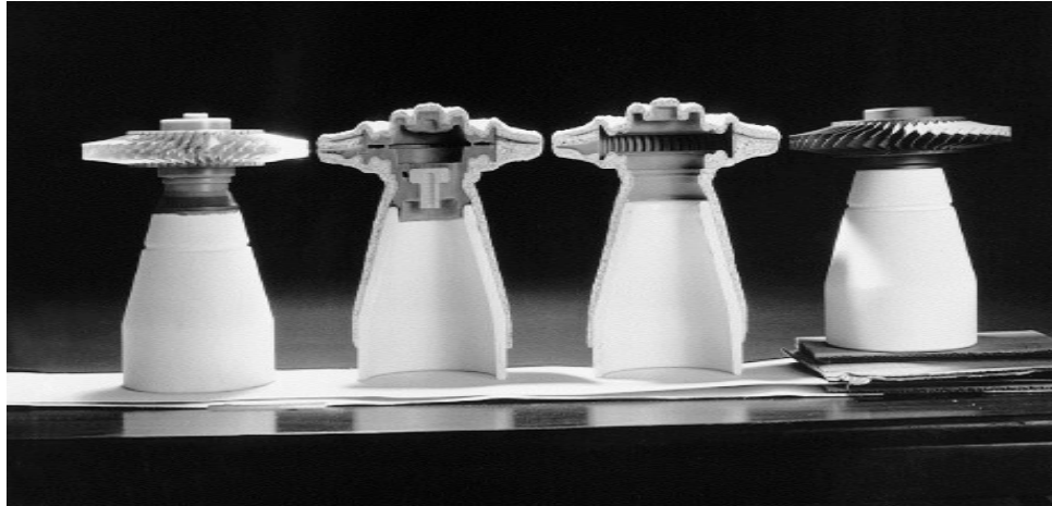
Investment casting of an integrally cast rotor for a gas turbine. (a) Wax pattern assembly. (b) Ceramic shell around wax pattern. (c) Wax is melted out and the mold is filled, under a vacuum, with molten superalloy. (d) The cast rotor, produced to net or near-net shape.
