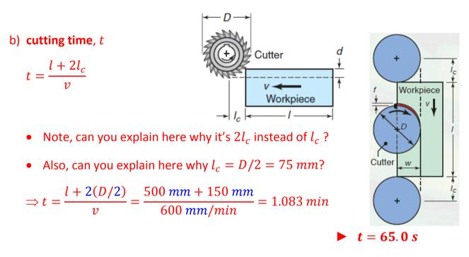
Let's test the above assumption. Just as with peripheral milling,  $l_c$  for face milling can be determined from the following formula (note how in face milling, d is replaced with w; compare the two figures above):
