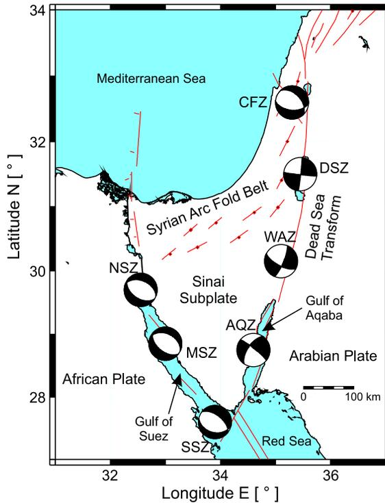
**Fig. 3.** The averaged fault-plane solutions derived from the moment tensor summation (Eq. (1)) for each seismogenic source, shown in Fig. 2. NSZ: North Gulf of Suez Zone, MSZ: Middle Gulf of Suez Zone, SSZ: South Gulf of Suez Zone, AQZ: Gulf of Aqaba Zone, WAZ: Wadi Araba Zone, DSZ: Dead-Sea Zone, CFZ: Carmel Fault Zone.
