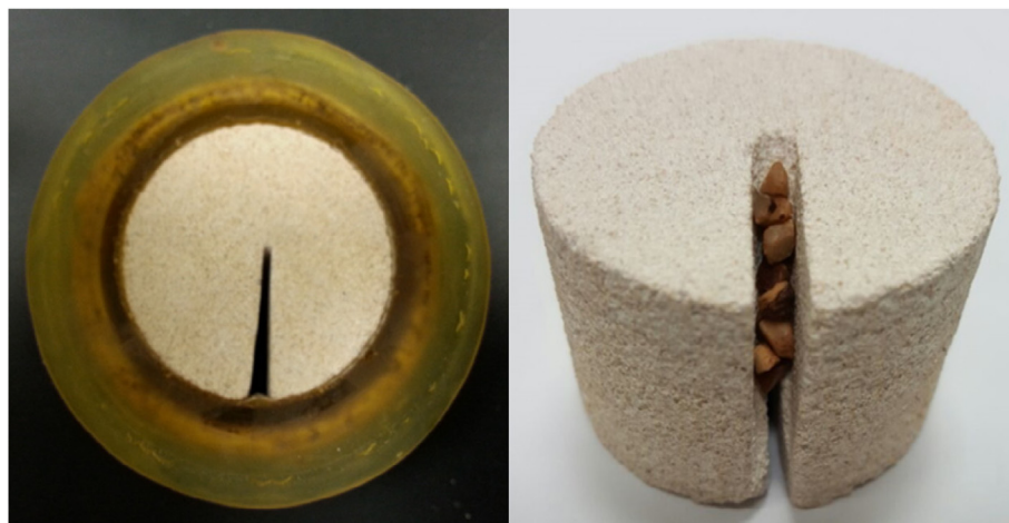
Fig. 6. Demonstration of the coarse date palm seeds trapping in the induced fracture.
