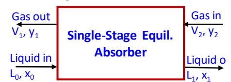
Figure 2: Equilibrium Single-stage Contacting
