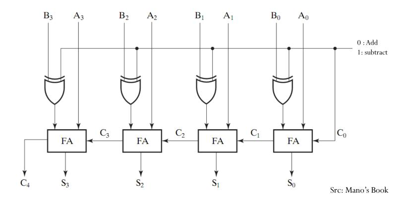
Using full adders and XOR we can build an Adder/Subtractor!
