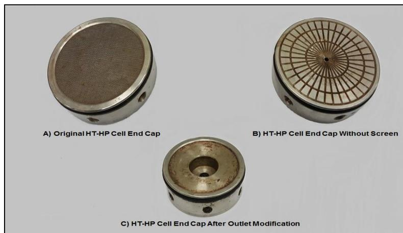
**Fig. 3- HT-HP filtration cell end cap before and after modification.**
