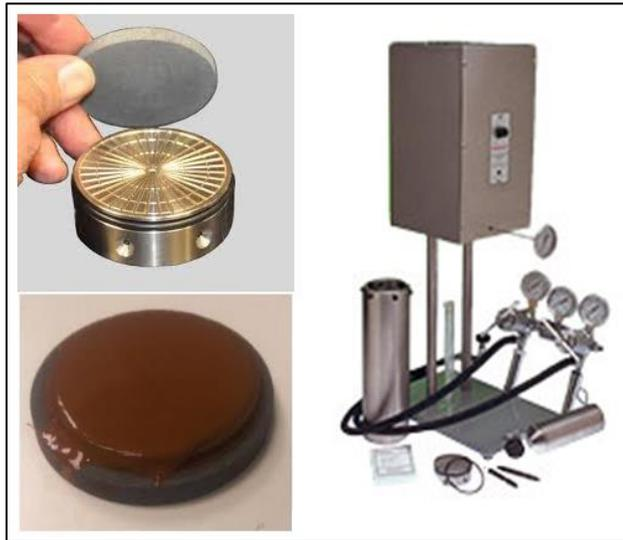
**Fig. 1- Standard HT/HP API filter press (500 ml).**
