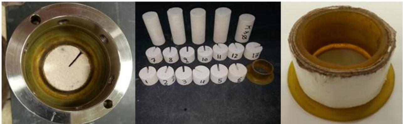
**Fig. 2- The developed core holder and the testing core plugs with fracture.**
