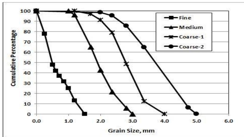
Fig 5- Grain size distribution of the tested crushed date palm seeds.
