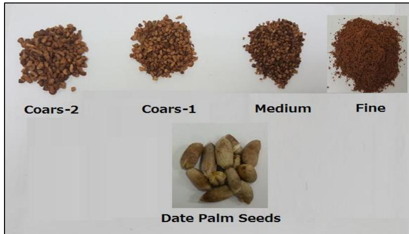
Fig 4- Grain sizes of the crushed date palm seeds.
