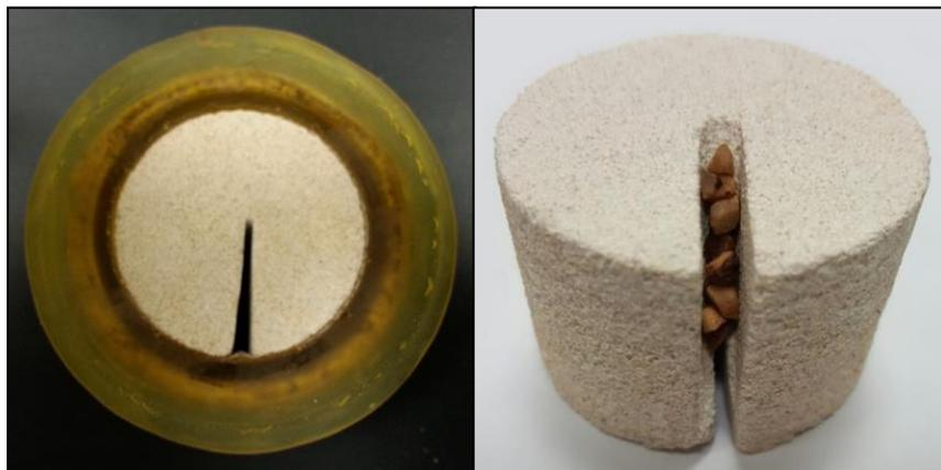
Fig. 6- Demonstration of the date palm seeds trapping in the induced fracture.
