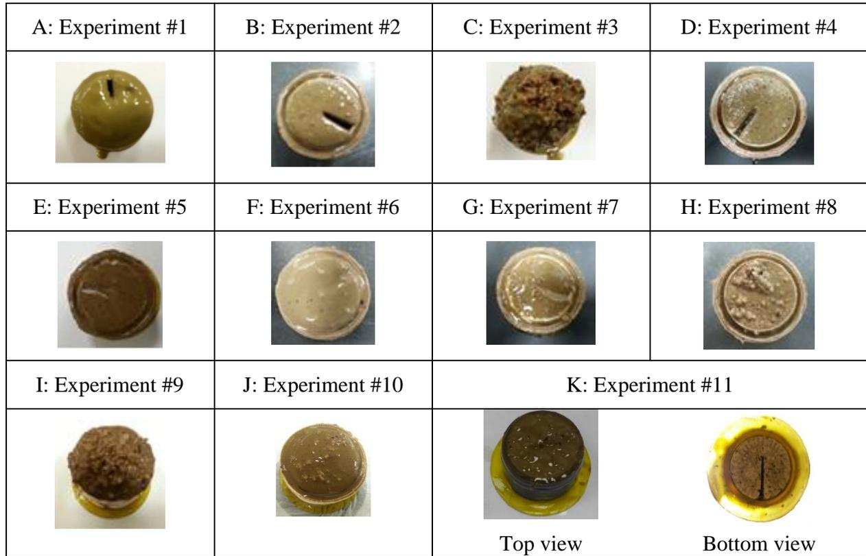
Fig. 7- The fractured sandstone core plugs at the end of experiments.
