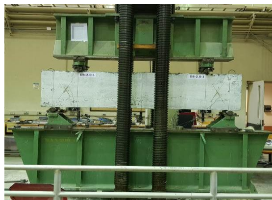
Fig. 5. Testing machines: the beam specimens using the AMSELOR ® hydraulic testing machine
