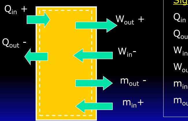
Sign convention Q<sub>in</sub> is positive Q<sub>out</sub> is negative W<sub>in</sub> is negative W<sub>out</sub> is positive m<sub>in</sub> is positive m<sub>out</sub> is negative
