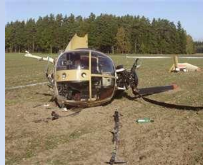
Helicopter Crash due to Engine Failure
