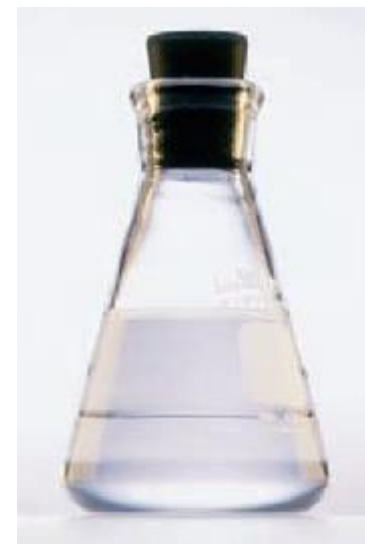
Hexane is insoluble in water (hexane is in the top layer because it is less dense than water).
