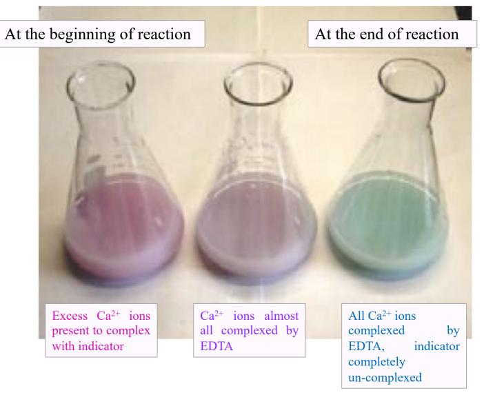
Figure 4. Color changes for calcium-EDTA titration
