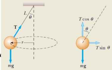
Example 6.2 The Conical Pendulum (continued)  $T \cos \theta = mg$   $T \sin \theta = ma_c = m \frac{v^2}{r}$   $\frac{T \sin \theta}{T \cos \theta} = \frac{m \frac{v^2}{r}}{mg} \Rightarrow \tan \theta = \frac{v^2}{gr}$   $v = \sqrt{gr \tan \theta}$  $r = L \sin \theta \Rightarrow v = \sqrt{Lg \sin \theta \tan \theta}$
