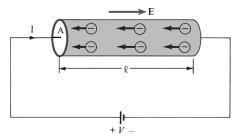
The current is defined as the rate at which charge flows through this surface. The SI unit of current is the ampere (A):
