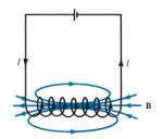
The magnetic flux is proportional to B, which in turn is proportional to the current in the circuit.
