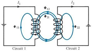
Let us take  $\Phi_{12}$  which is the flux passing through circuit 1 due to current  $I_2$  in circuit 2.
