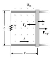
When an applied force  $F_{app}$  moves the bar to the right with a velocity v, the free charges in the wire experience a magnetic force directed along the length of the bar. This force creates motional electromotive force that causes an induced a counterclockwise current I in the loop.
