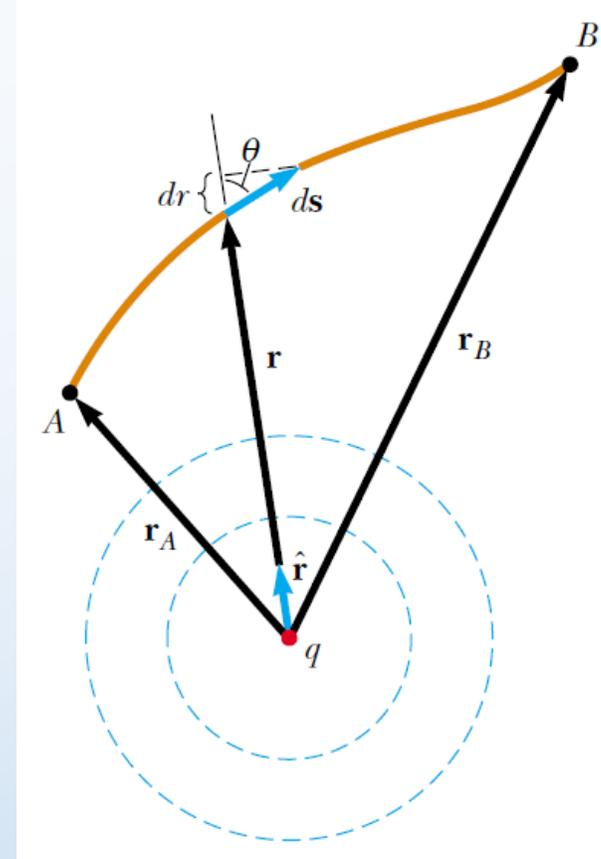
The potential difference between points  $A$  and  $B$  due to a point charge  $q$  depends only on the initial and final radial coordinates  $r_A$  and  $r_B$ . The two dashed circles represent intersections of spherical equipotential surfaces with the page.
