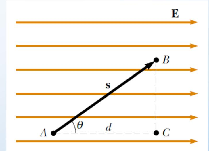
A uniform electric field directed along the positive  $x$  axis. Point  $B$  is at a lower electric potential than point  $A$ . Points  $B$  and  $C$  are at the same electric potential.
