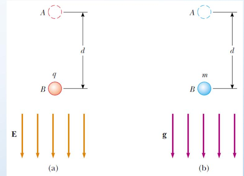
(a) When the electric field  $\vec{E}$  is directed downward, point  $B$  is at a lower electric potential than point  $A$ . When a positive test charge moves from point  $A$  to point  $B$ , the charge–field system loses electric potential energy. (b) When an object of mass  $m$  moves downward in the direction of the gravitational field  $g$ , the object–field system loses gravitational potential energy.
