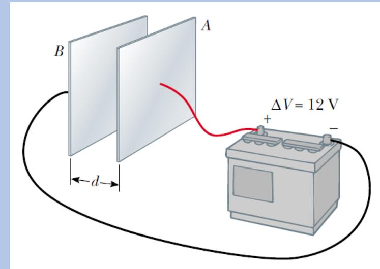
A 12 V battery connected to two parallel plates. The electric field between the plates has a magnitude given by the potential difference  $\Delta V$  divided by the plate separation  $d$ .
