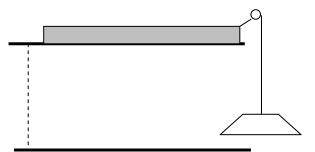
An 18 kg slab slider show a 15° in clinked plain on 3- mm think film of oil at 20 C (  $\mu$  = 8.14 E - 2 N.S/m2 ) contact area is 0.3 m2 find the terminal velocity of the slab ?
