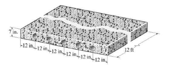
$$W = (144 \text{ lb/ft}^3)[(12 \text{ ft})(6 \text{ ft})(\frac{7}{12} \text{ ft}) - 5(12 \text{ ft})(\pi)(\frac{2}{12} \text{ ft})^2] = 5.29 \text{ k} \qquad \text{Ans}$$
