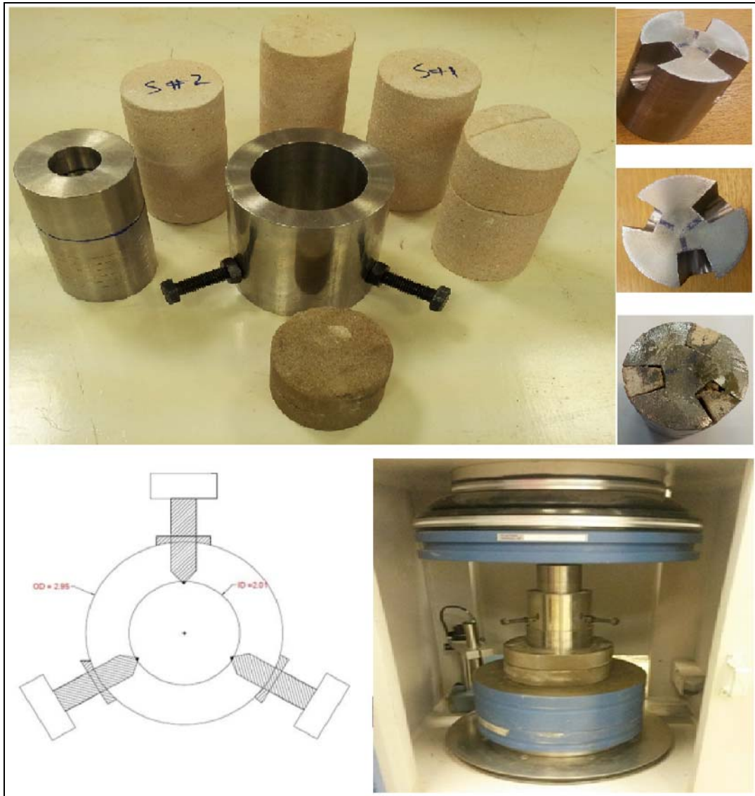
Fig. 4. Details of rock scratching cell developed in this study.
