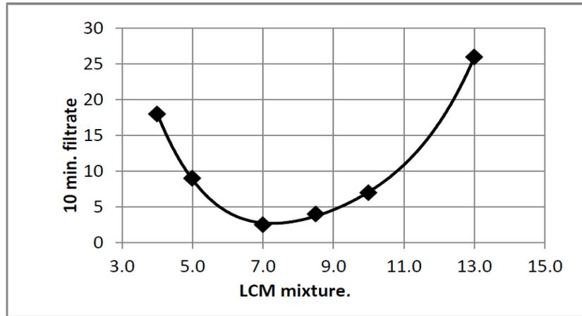
Fig. 11. Relationship between FSM weight percent and 10 min filtrate volume.
