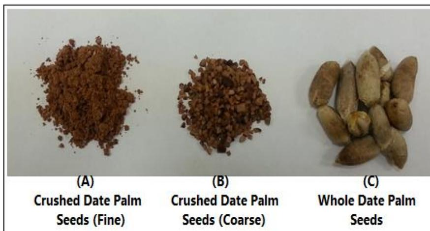
Fig 5. Grain sizes of the crushed date palm seeds.
