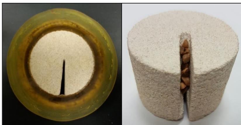
Fig. 9. Demonstration of the date palm seeds trapping in the induced fracture.
