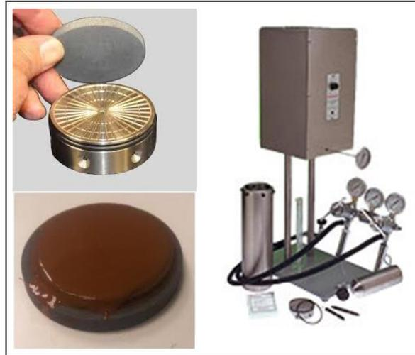
Fig. 1. Standard HT/HP API filter press (500 ml), After Fann Instrument Company, USA.
