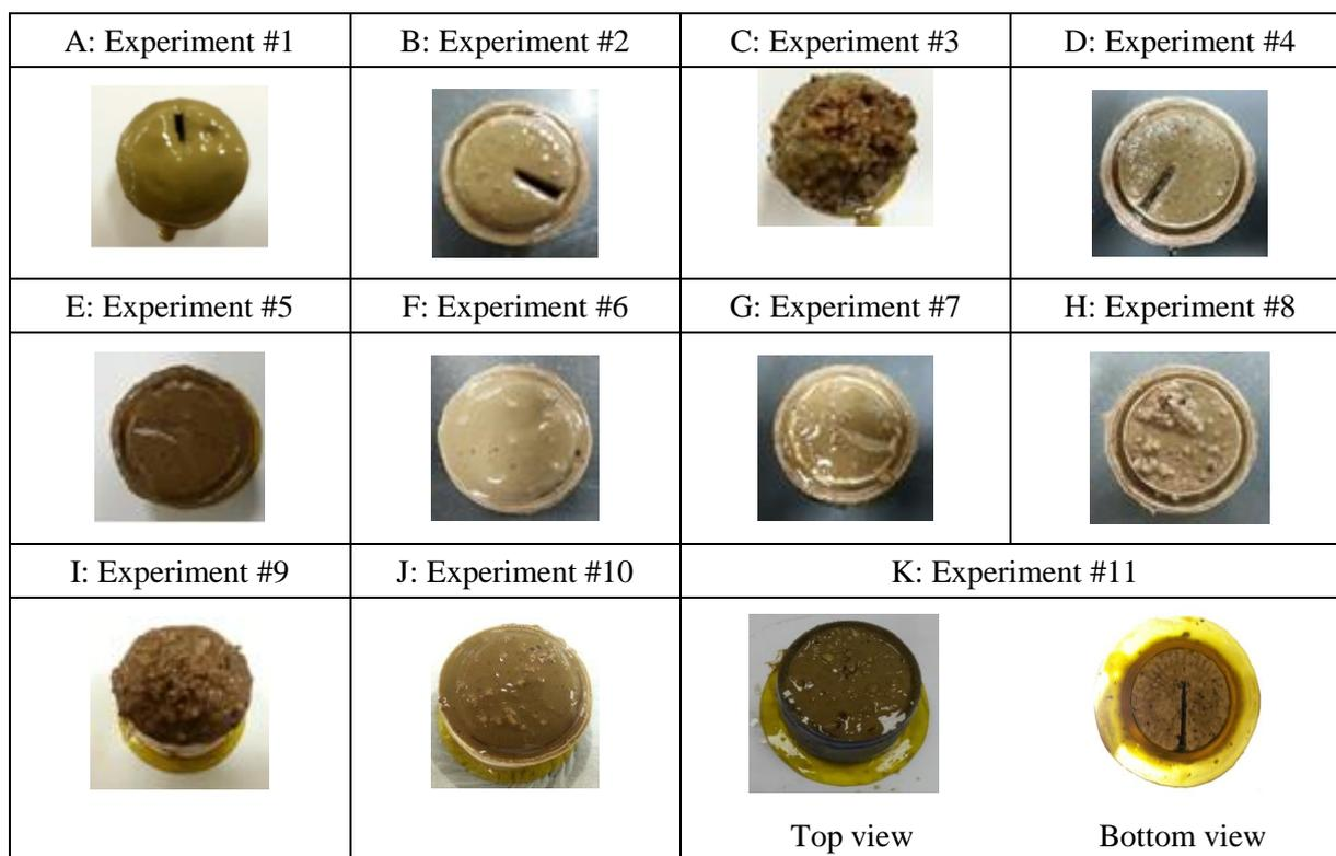
Fig. 10. The fractured sandstone plugs at the end of experiments using crushed date palm seeds.
