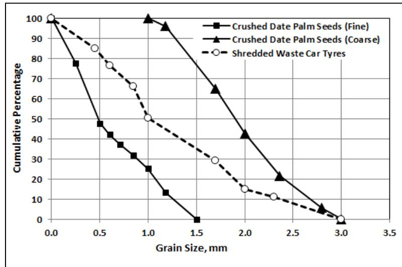
Fig 6. Grain size distribution of the tested fracture seal materials.
