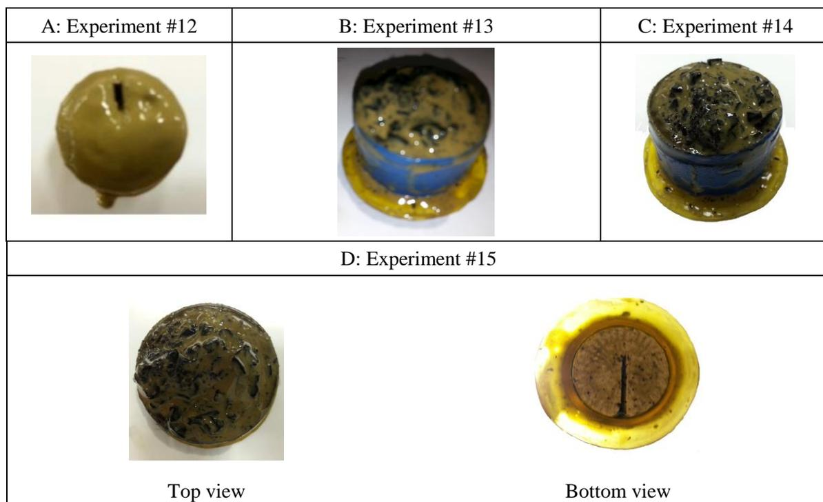
Fig. 14. The fractured sandstone core plugs at the end of experiments.
