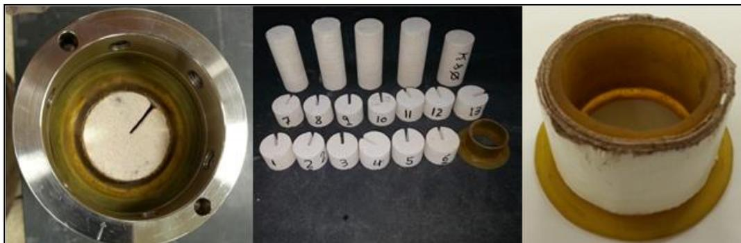
Fig. 2. The developed core holder and the testing core plugs with fracture.
