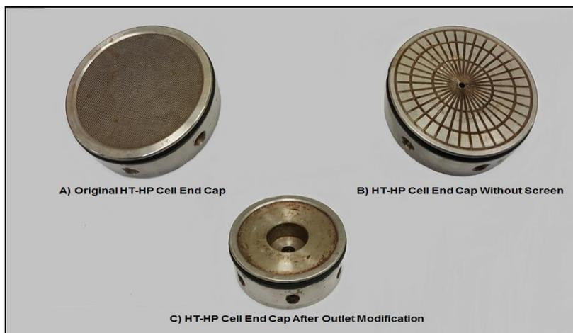
Fig. 3. HT-HP filtration cell end cap before and after modification, After Fann Instrument Company, USA.
