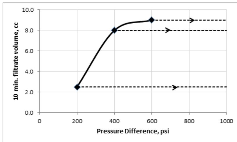
Fig. 13. Relationship between pressure difference and spurt volume at 25°C.
