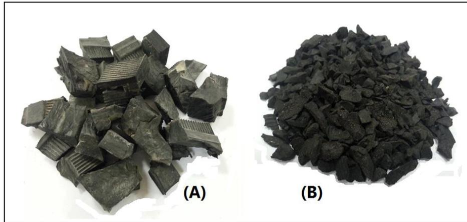
Fig. 8. Shredded car waste tyre pieces before (A) and after crushing (B).
