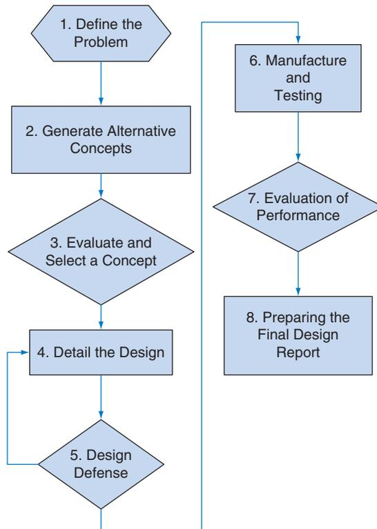
**FIGURE 17.1** The Design Process Flowchart
