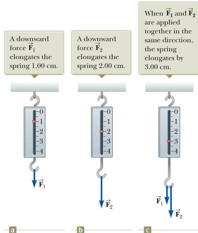
A spring can be used to calibrate the magnitude of a force.
