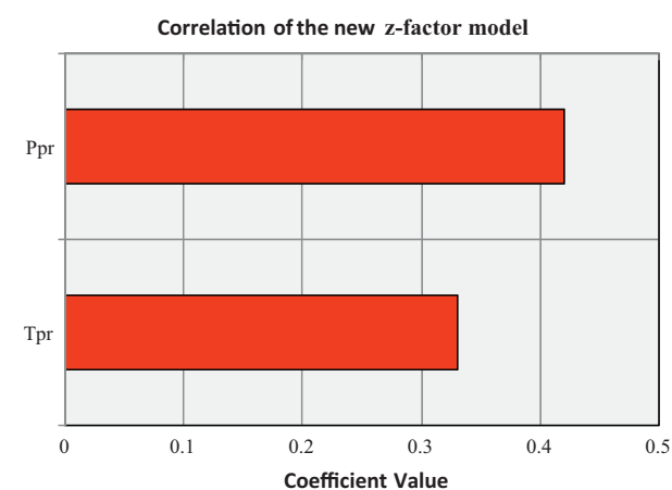
Fig. 8 – Sensitivity analysis of the new z-factor model and its dependence on each independent variable.
