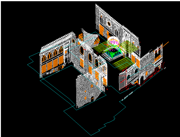
Figure 6 3D reconstructions of the building; drafted elevations are tied to one coordinate system with the help of the plan profile captured by total station. (ECAE, 2005)
